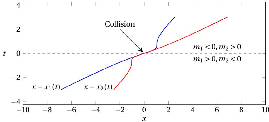
Figure 11: Spacetime plot showing the locations  $x_k(t)$  of the peakons in the  $(x, t)$ -plane for the peakon–antipeakon solution in Figure 10 with  $\lambda_1 = 1/2$ ,  $\lambda_2 = 1$  and  $b_1(0) = -b_2(0) = \sqrt{3}$ . Note how the curves approach the straight lines  $x = t/\lambda_k + \text{const.}$  given by (4.28) as  $t \rightarrow \pm\infty$ , and that both curves are tangent to the line  $x = (1/\lambda_1 + 1/\lambda_2)t = 3t$  at the origin, in agreement with (4.29).
