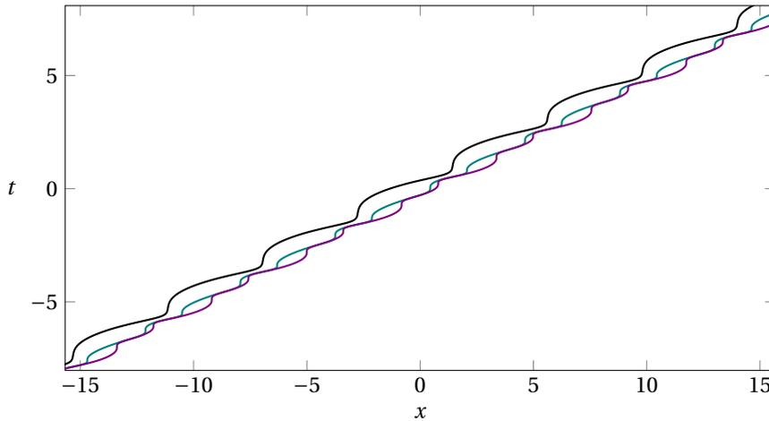
Figure 25: Positions  $x = x_k(t)$  for the 3-peakon solution obtained using the eigenvalues  $\lambda_{3,4,5}$  from (5.19) together with the modified residues  $b'_{3,4,5}(0)$  from (5.21). This 3-peakon solution looks just like the 3-peakon cluster seen in Figure 22 as  $t \rightarrow +\infty$ , in agreement with Theorem 5.25.
