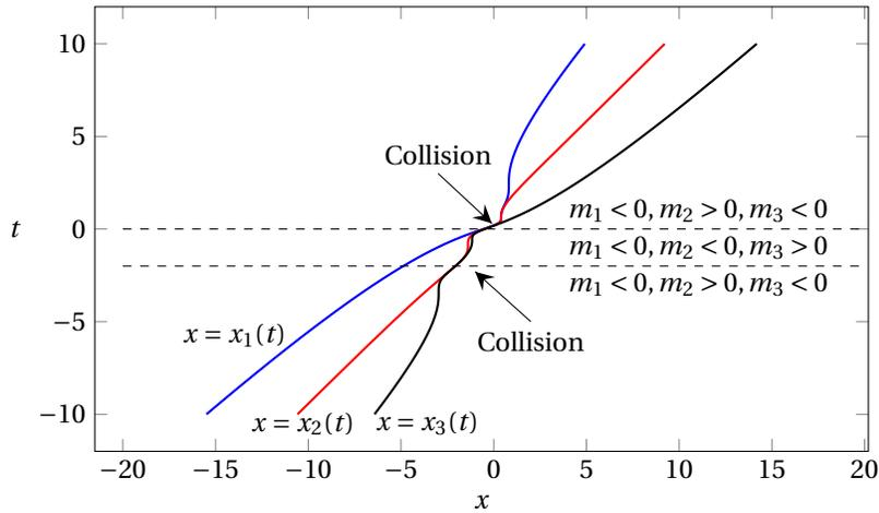
Figure 27: Spacetime plot showing the locations  $x_k(t)$  of the peakons in the  $(x, t)$ -plane for the peakon–antipeakon solution with a triple eigenvalue  $\lambda_1 = \lambda_2 = \lambda_3 = \mu$ . The parameters used here are  $\mu = 1$  and  $b_1(0) = b_2(0) = 0$ ,  $b_3(0) = -1$ . In this case, there are no collisions between  $x_1$  and  $x_2$ , but  $x_2$  and  $x_3$  collide twice (when  $t = -2$  and  $t = 0$ , according to Theorem 6.32).
