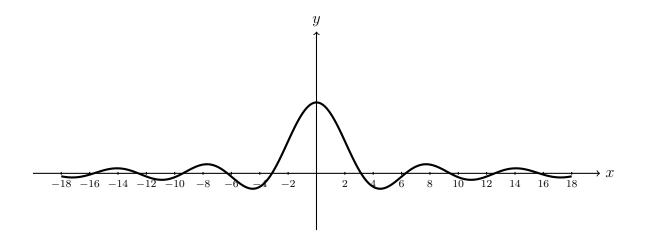
Show that the Fourier transform of u(x) = 1,  $x \in [-1, 1]$ , and u(x) = 0 elsewhere, is given by  $U(\omega) = 2 \operatorname{sinc} \omega$ .
